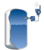
Wireless applications using a Rosemount 702 Wireless Discrete Transmitter
