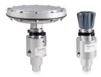
The 50-4000 Series accurately controls high-pressure water glycol while decreasing pressurization time and extending regulator life. Units feature an integrated bypass valve that controls large variations in flow rates at pressures up to 15,000 psiq.
