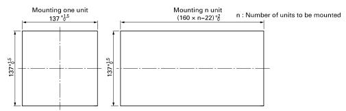
Do not use the water proof packing in case of mounting n unit
