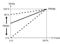
In the case of a suction throttle valve, it is essential that a minimum stroke limit be maintained to ensure compressor cooling and efficient oil return. This can be achieved with a reinjection valve, a bypass line across the valve, or a guaranteed minimum opening of the valve. The minimum stroke can be defined via the controller and control signal Y, or it can be set directly with potentiometer Rv.
