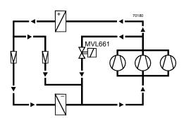
Suitable for large refrigeration systems in air conditioning applications with several compressors or compressor stages, and where the evaporator and compressor are some distance apart (attention must be paid to the oil return).
