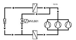
Suitable for use in large refrigeration systems in air conditioning plant, to prevent unacceptable temperature fluctuations between the compressor stages.
