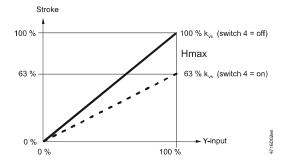
For  $k_{VS}$  reduction (DIL switch 4 in position ON), the stroke is limited to 63% mechanical stroke. 63% of full stroke then corresponds to an input/output signal of 10 V. If, in addition, the stroke is limited to 80%, for example, the minimum stroke is 0.63 x 0.8 = 0.50 of full stroke.
