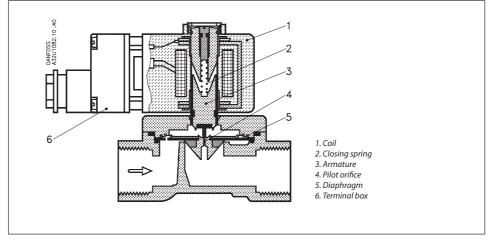
Proportional regulation of the opening and closing of the EV260B valves is achieved through stepless regulation of the coil current and thus of the pulling force of the solenoid coil.
