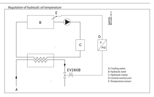
To control viscosity and thus friction, it is important to keep a constant oil temperature in hydraulic motor (C). Cooling is therefore often required.
