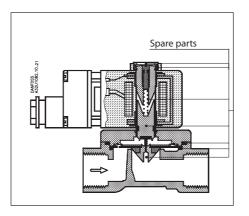
The spare parts kit comprises e.g. a locking button and nut for the coil, armature with valve plate, spring, O-rings and diaphragm.
