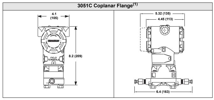
(1) For FOUNDATION fieldbus and Profibus PA transmitters with LCD Display, housing length is 5.78 in. (147 mm).
