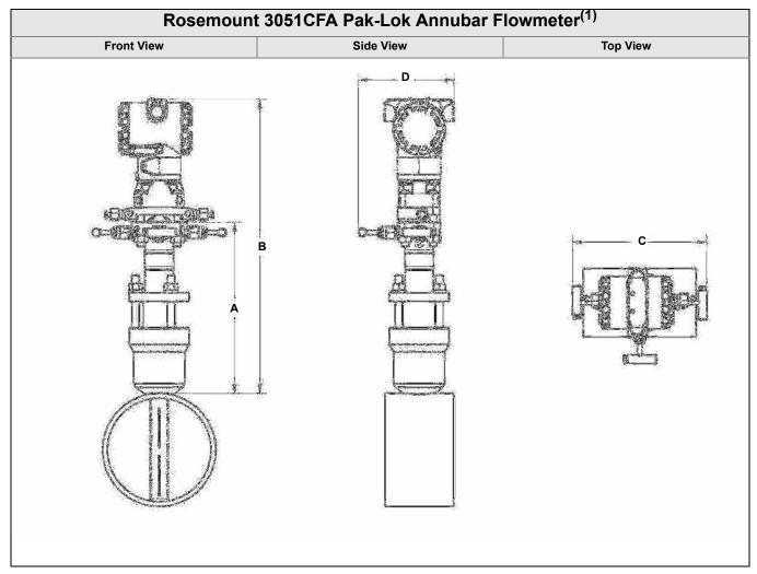
(1) The Pak-Lok Annubar model is available up to 600# ANSI (1440 psig at 100 °F (99 bar at 38 °C)).
