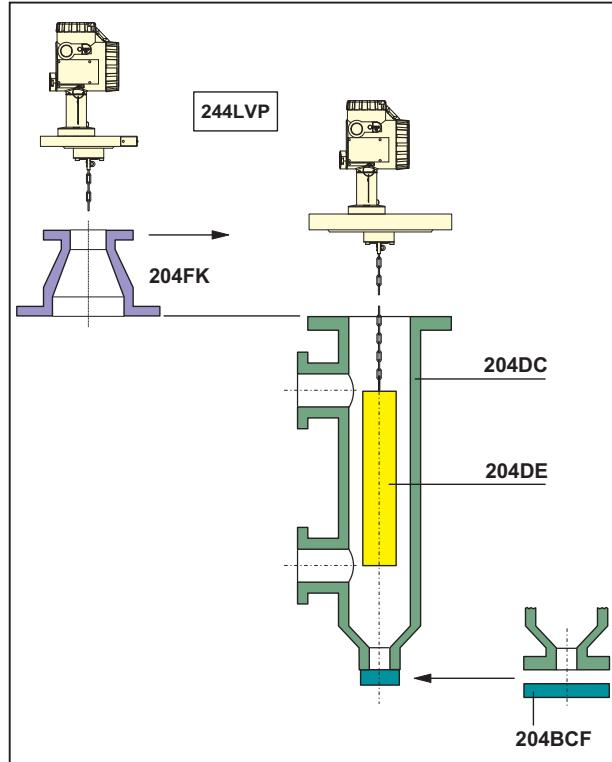
**MODEL CODES 204DE****Displacer for Buoyancy Transmitters from 2N buoyancy up to 20N 204DE**
