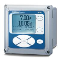
Rosemount 1056 Dual Channel Transmitter is a line powered device that can accept inputs from pH/ORP, ISE, flow, conductivity (contacting and toroidal), turbidity, and amperometric (dissolved oxygen, chlorine, and ozone) sensors.
