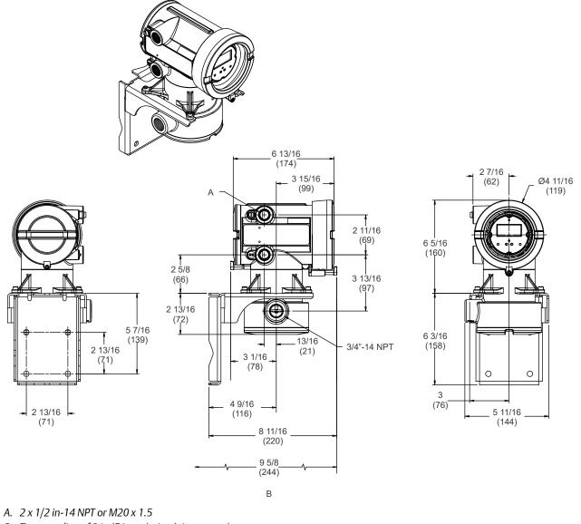
B. To center line of 2 in (51 mm) pipe (pipe mount)
