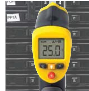
Spot pyrometer, temperature measurement in one spot.
